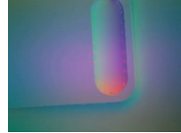
Figure 9. Insert USB: verifying object progress. Seed 10066, V+T, success. The connector remains exposed while the tactile contacts shift, and the action note identifies finger slip along a blocked plug. Astra withdraws, recenters, and issues a submillimeter correction before insertion progresses. Hand motion is not treated as sufficient evidence that the connector has entered the socket. Full rollout .
